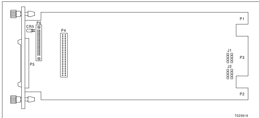
Figure 3-5. IMMPIO1 Board Layout
